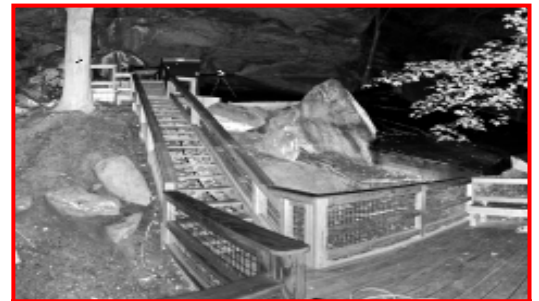
Quantapoint 2D Laser Scan (Not a Picture) Each Point is a Measurement
